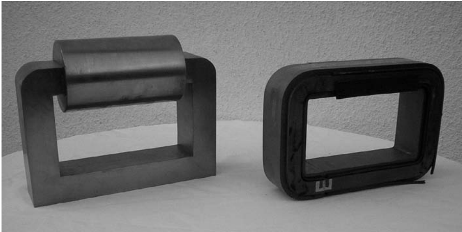
Figure 4. Simplified experimental transformer core with a solid coil and its original counterpart
